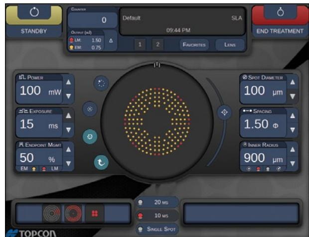
Figure 3. The screen of the PASCAL Laser System with Endpoint Management software. The central pattern shows landmark spots in red, while endpoint spots are shown in yellow. Endpoint power is approximately half of the power used for landmarks.
