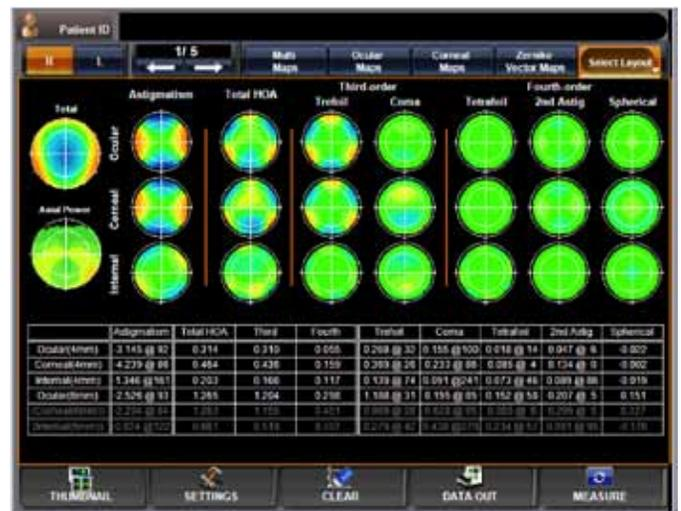
**Figure 3:** The KR-1W features a component map display which shows the high order aberrations for the entire ocular system.
